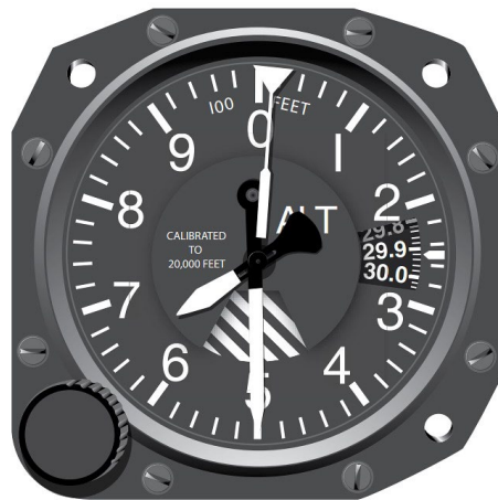
This altimeter reads 6,500 feet MSL. The altimeter setting / barometric pressure is set for 29.92. Courtesy FAA.
