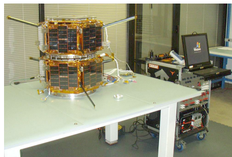
Fastrac 1 and 2 undergoing final electronic testing prior to launch (Courtesy: University of Texas at Austin)
