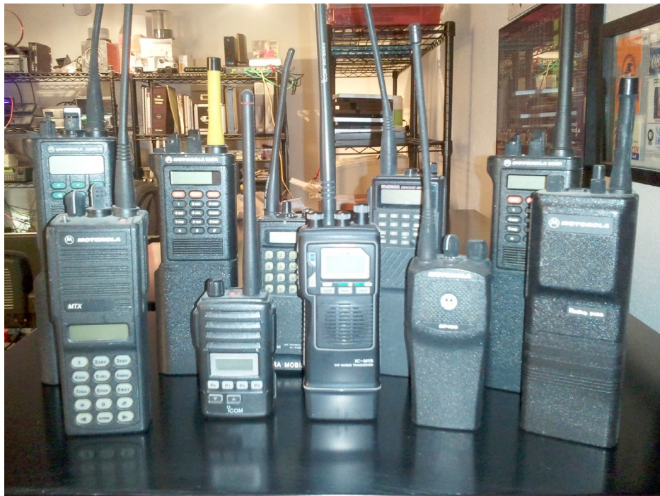
An assortment of professional-grade public service band radios. A more sensitive receiver and better quality audio come with a price: Hard to program, not necessarily all the bands you want to hear and may not be frequency agile. (Courtesy: Author)
