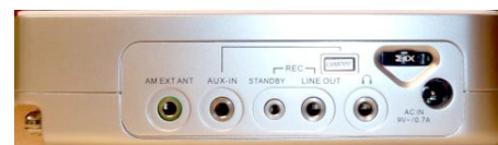
Lots of audio interconnect possibilities, an external AM antenna jack, and an RF gain control.
