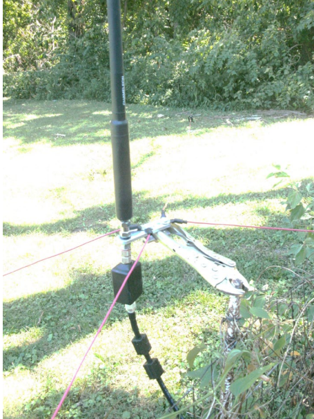
A close-up of the mounting, showing the counterpoise wires, the unun, and the clip-on ferrite beads. (Photo by author)
