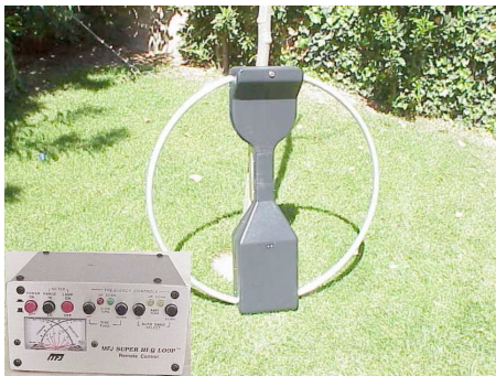
MFJ's Model 1786 magnetic loop and remote control box, shown at ground level for photo purposes only, offers continuous coverage of 30 through 10 meters (ham and SWL) with a single, compact antenna.
