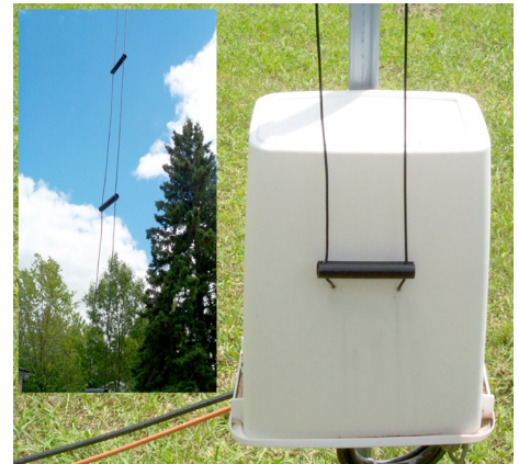
Figure 2 - The author's "pre condo" loop was tuned with a backyard autotuner on 160-6 meters. At the lower left you can see the 100-foot run of RG-8 coax and a large extension cord (used to provide 12-V dc to the tuner). The autotuner lived inside the garbage can weather shelter, which was U-bolted to a short pipe, and a 35-foot length of open-wire line went straight up to the loop's feed point (inset photo). Placing the tuner in the backyard eliminated RFI from the shack PCs and made the tuner available for occasional use elsewhere (it would have been a pain to retrieve it if it were mast-mounted at the loop's feed point)-NT0Z
