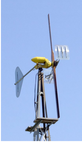
Refurbished 32 volt Wincharger in operation today. (Courtesy: Terry Bryant www.wincharger.com )
