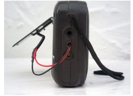
Side view shows power wires going into the radio cover.
