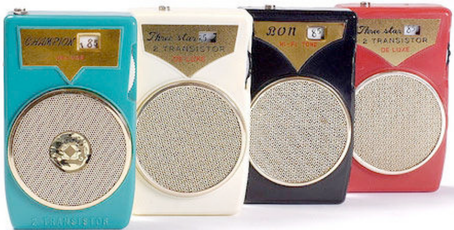
4 “Boy’s radios”, all inspired by the design of the Sony TR-610. These radios utilized a 2 transistor circuit and, classified as toys, were able to get around new U.S. tariffs against imported transistor radios.
