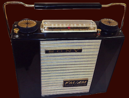
Sony TFM-151: Claimed to be the first solid state radio with FM cost $150 in 1958
