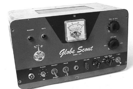
Fig. 1. Construction of the Globe Scout 680 is sturdy and compact. It weighs in at 25 pounds.
