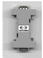
Figure 2 The RadioCom switchbox is a hardware form of copy protection called a “dongle.”
