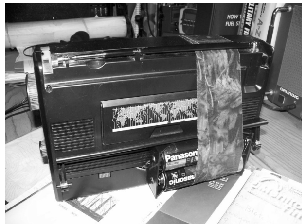
How to make a good radio UGLY: leave the batteries in for an extended period of time.
