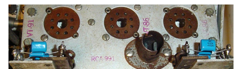
The r.f. and converter tube shelf with six new capacitors (three on each side) installed on the old terminal lugs.
