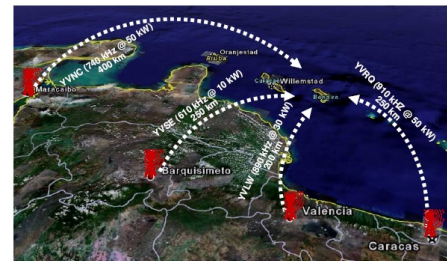
Signal-levels from over one hundred AM stations in Venezuela were monitored from Bonaire and normalized to 100 kW on 800 kHz.
