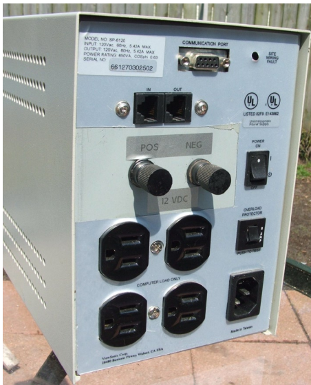
A UPS unit may be modified to provide 12 VDC from the batteries to power your radio in a power outage
