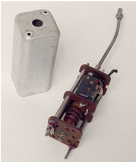
The c.w. oscillator module removed from its can. Original paper capacitor still in place. The flexible cable at the top connects with the front panel bfo control.
