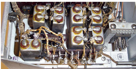
The bank of 0.5 mfd paper bathtub capacitors. After doing some testing, I'm hoping that all might still be ok.
