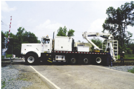
Norfolk Southern Brandt unit getting off the rails at a road crossing. Note that the unit is equipped with a hydraulic arm that can be used either as a lightweight crane or as a cherry-picker to lift personnel to work on lineside equipment.
