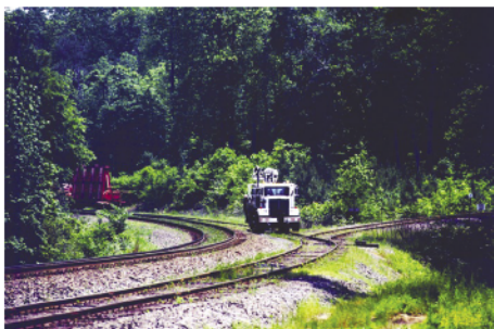
A Norfolk Southern Brandt unit has set out now empty cars used to deliver track components and is heading to the next road crossing to get off the tracks.
