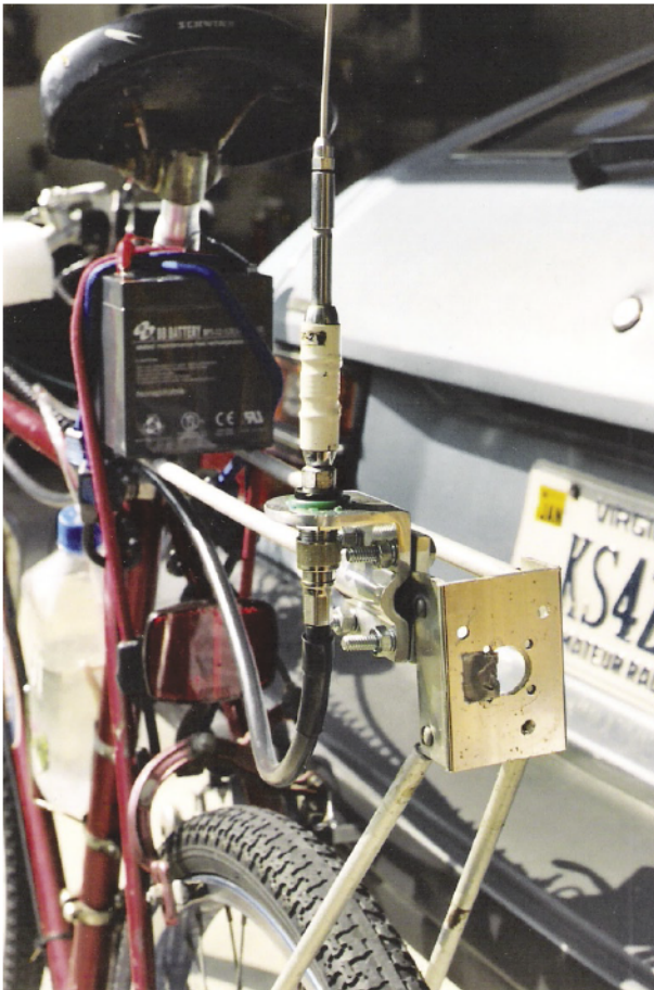
Close-up of antenna support with 2 meter 5/8 wave antenna. To get the full 5 watts output for the 1 hour daily trip I power the HT from a small trailer light battery I found at an auto supply store for under $10. It's visible in the background under the seat. (Courtesy: Author)
