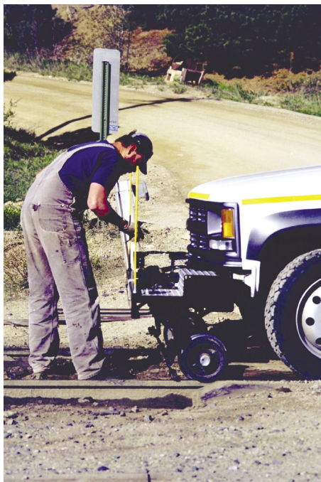
A Union Pacific employee in Colorado locks down the flanged guide wheels on his hi-rail truck.
