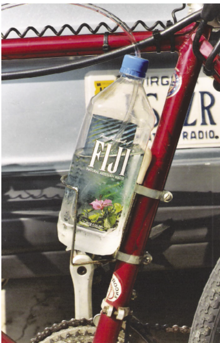
Berger Bottle in bottle holder. To make your own: Drill a hole in the plastic bottle cap big enough to insert clear tubing to the bottom of the bottle. Drill a small breather hole next to the tube hole to equalize air pressure inside the bottle. The drinking end of the tube is secured to the handlebars with a tie-wrap. I used a Fiji water bottle because it fit nicely into the water cage and already had water in it when I bought it! (Courtesy: Author)
