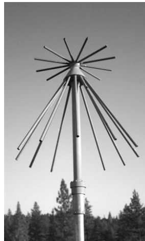
The military surplus discone AT-197A/GR, 225-400 MHz, is coveted by some Mil listeners. This particular one is rebuilt with an "F" connector way up inside.
