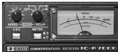
Figure 2 – Icom R7000 S-Meter used to compare signal strengths.
