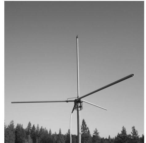
Figure 3 – Reference quarter-wave VHF Ground Plane with horizontal radials and impedance matching section.
