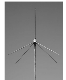
Quarter-wave Ground Plane with sloping radials. Radials 23 inches from antenna center. Vertical element 23 inches from insulator base.
