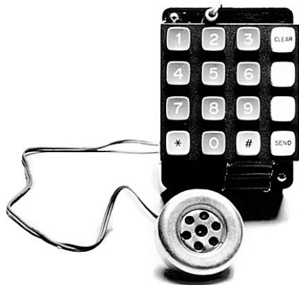
2600 referred to the idle tone that would make tandem switches in long-lines offices disconnect and await further instructions. Pictured is Steve Wozniak’s original “blue box,” now in a computer museum.
