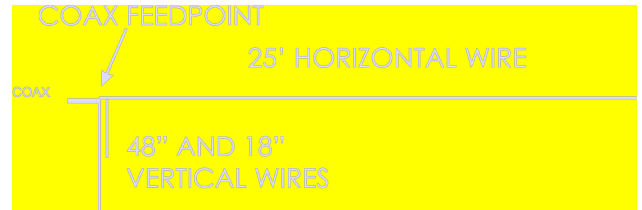
A 25-foot horizontal wire with two short wires (18" and 48") dangling from the left end. The center wire of a coax cable is soldered at that mutual point.
