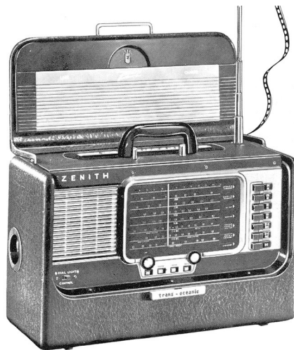
A 600 series Trans-Oceanic. The Waverod telescoping antenna is extended and the Wavemagnet has been removed from its slot at the top of the case. Its cord extends upwards at the top right.
