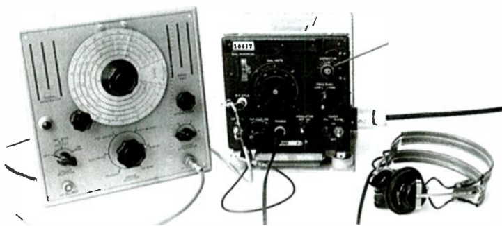
The 2432 hooked up the Navy "LM" for testing. Headset allows signal from the 2432 to be adjusted to "zero beat" with signal of precise frequency generated internally in "LM."
