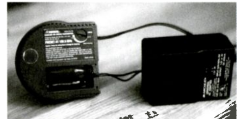
Soldered alligator clips take the place of batteries and provide drift-free long term operation. Imagine the number of batteries I'd have gone through in the last six years!
