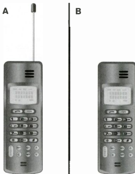
FIG. 1. (A) A "last century's" cellphone with a short whip antenna, and (B) a 21st century cellphone with an embedded antenna. (Can't see the antenna? That's the point.)
