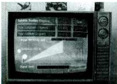
PHOTO 5: Pressing "set up" on the main menu brings up a screen showing where to point the dish for reception and a handy signal meter which indicates signal strength. Photo Courtesy: Ken Reitz
