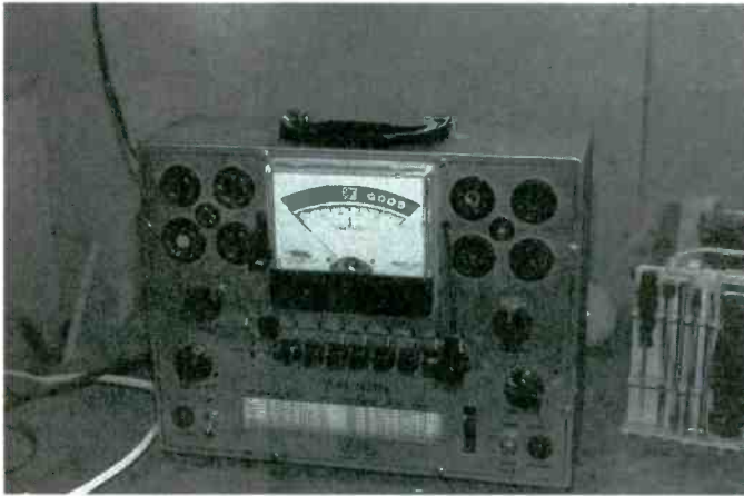
An old Eico tube tester. The scroll at the bottom contains the settings needed to test individual tubes.
