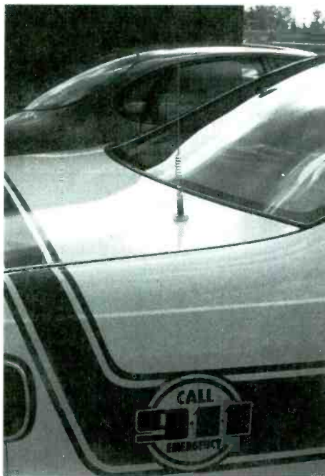
An 800 MHz antenna used on the Harris County trunked system
