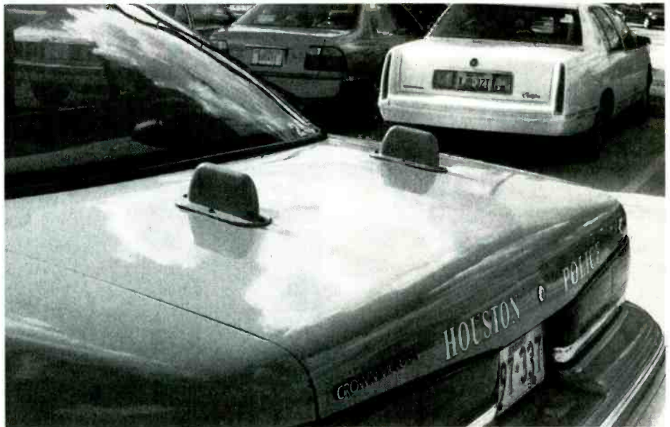
These two antenna covers hide antennas for 460 MHz communications and an 800 MHz mobile data terminal. But they didn't fool the frequency counter.
