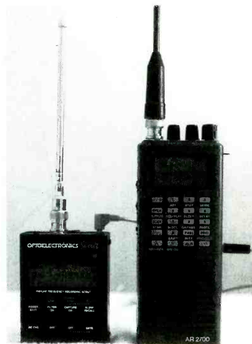
Some scanners can be automatically tuned by a sophisticated frequency counter.
