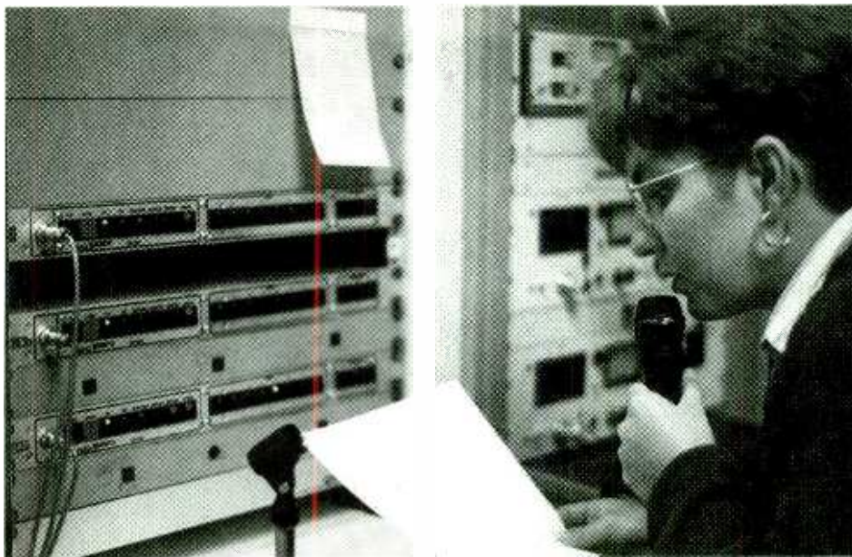
Hydrometeorological Technician Christy Smith records the latest weather announcement for one of four NOAA Weather Radio Stations under Wakefield's direction. The three units in the rack at the left are digital audio consoles. Each one replaces the gear in the rack to the right.
