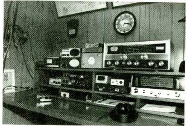
The shack of K7YHA consists of 45% recycled equipment. Top shelf L to R: Rotor control box, two Bearcat scanners, MFJ packet radio and TNC atop speaker, Hallicrafters SX-130 HF receiver. Bottom shelf: MFJ antenna tuner, Ten-Tec Argonaut 515 QRP transceiver, digital readout for the Argonaut and power supply, two active audio filters, and a Heath GR94 SW receiver.
