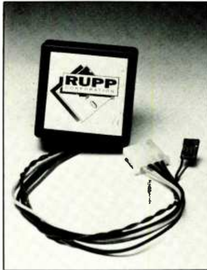
Rupp Corp.'s bAT Pak self-recharging battery for IBM AT and compatible computers plugs into a standard disk-drive power connector and the external battery connector on the motherboard. Its rated life is 10 years.
