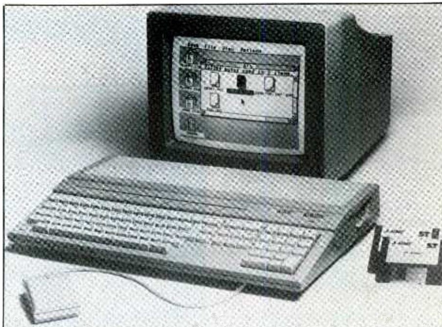
Atari's 1040STF computer has an 8-MHz 68000 microprocessor, 1 MB of RAM, 192K of ROM, built-in 3.5-inch floppy drive and a port for adding a 20-MB hard disk.
