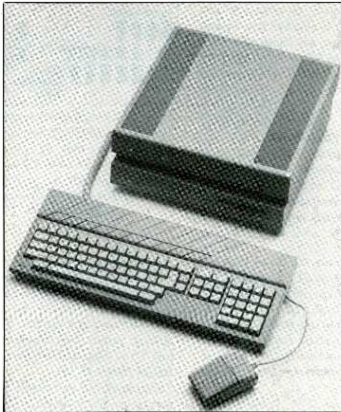
The Atari Mega uses an 8-MHz Motorola 68000 microprocessor. It comes with either 2 MB of RAM (Mega 2) or 4 MB of RAM (Mega 4), 192K of ROM, built-in 3.5-inch floppy drive, keyboard and mouse.
