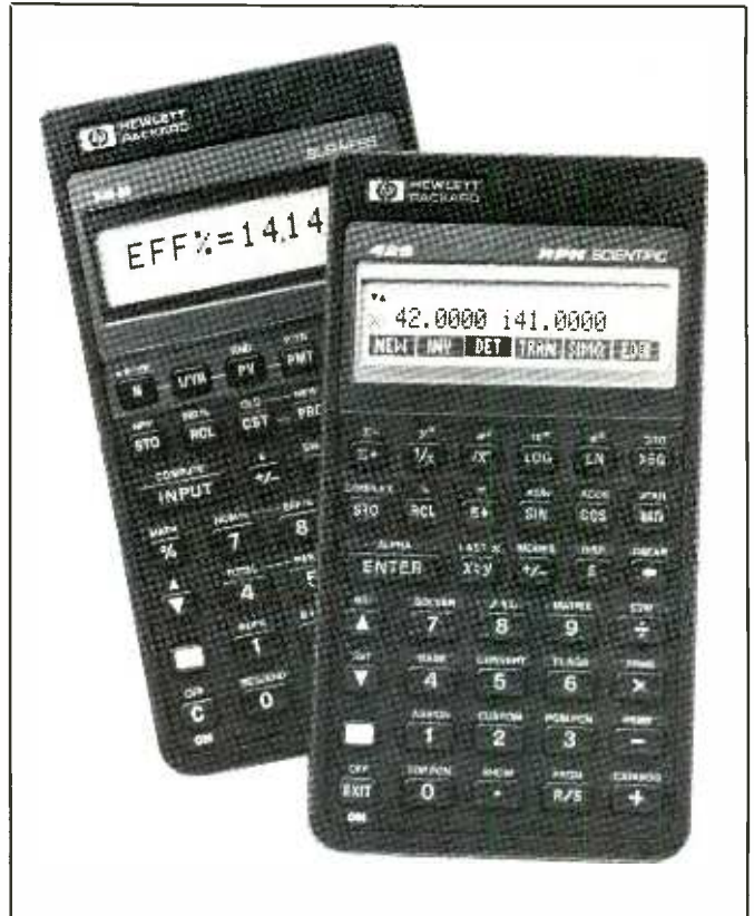
The HP-14B (left) gives business students and professionals the ability to label values for easy identification, while the HP-42S (right) RPN scientific calculator for engineers displays complex numbers in the same way they are written on paper.
