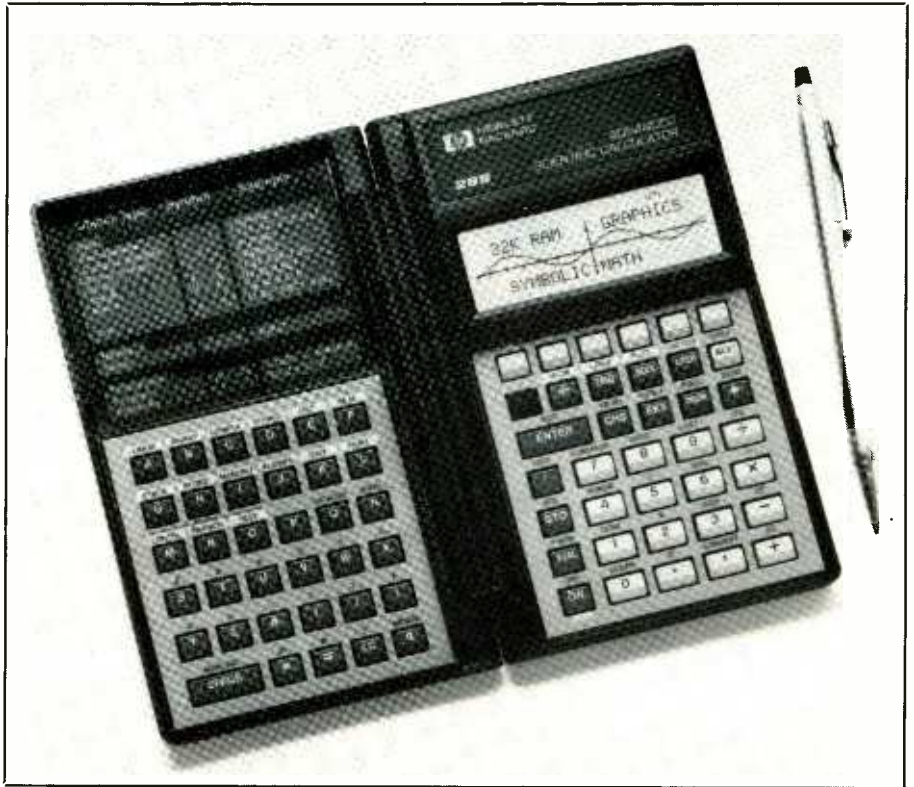
The HP-28S is Hewlett-Packard's top-of-the-line scientific calculator. It can solve symbolic algebra and calculus problems and graph multiple equations in its large liquid-crystal display window.
