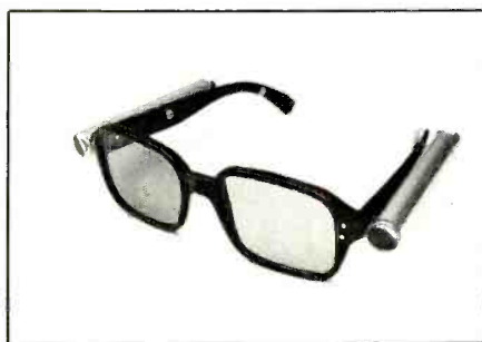
Fig. 7 Author's eyeglass-mounted infrared travel aid for the blind.
