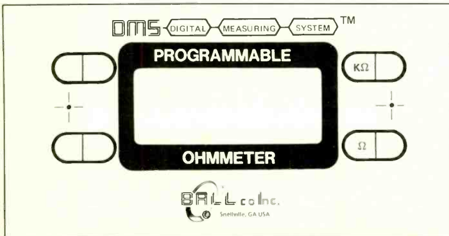
Fig. 8. Actual-size front-panel inlay artwork to use when Digi-Ohm module is attached to DMS module.
