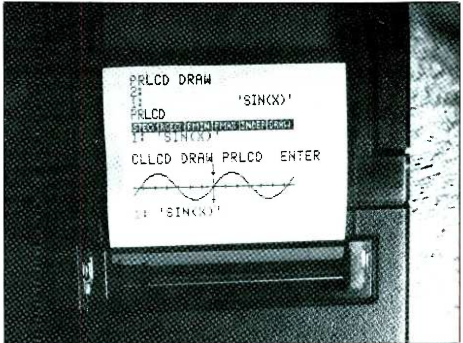
A graph was plotted on a 28C calculator and printed on H-P's $135 printer, as shown. Printing directions can be sent with up to a foot and a half separation between the 28C and the printer with no cord connection, providing a user with a hard copy record of his calculations.
