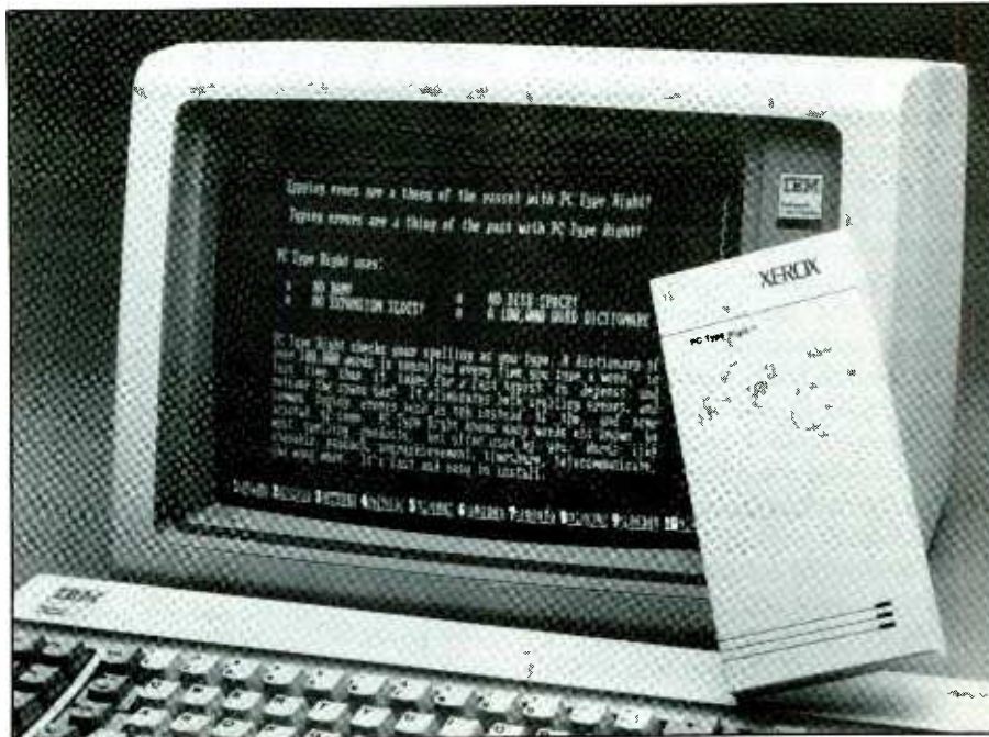
Xerox' PC Type Right from Microlytics, Inc. checks your spelling as you type with a dictionary of over 100,000 words. The outboard device connects between the keyboard and the computer's keyboard receptacle, using no disk space, random-access memory or expansion slot.
