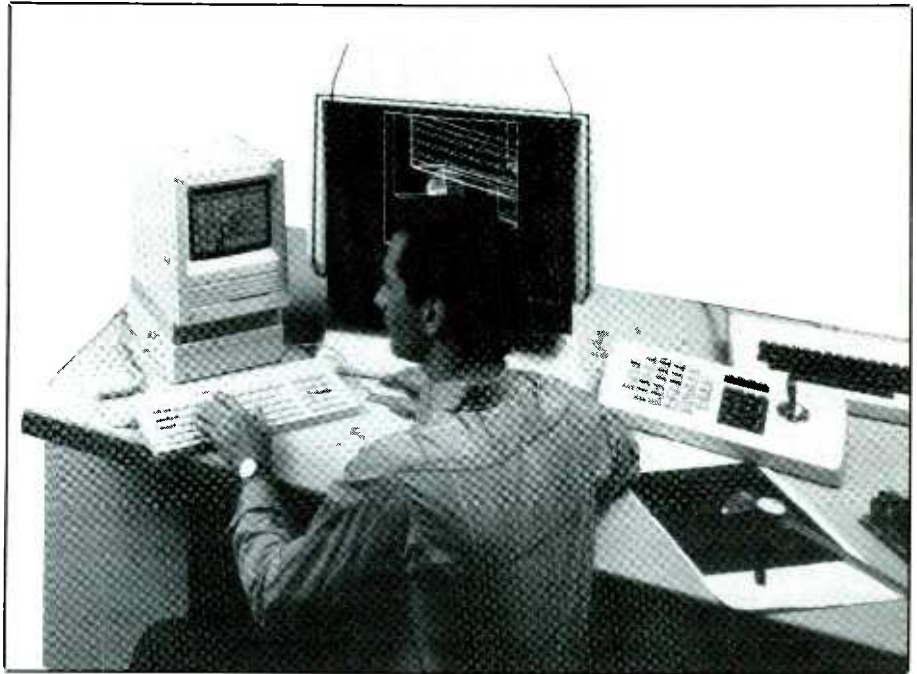
Mac's SE bus and Accessory Port permit use of large-screen monitor.
