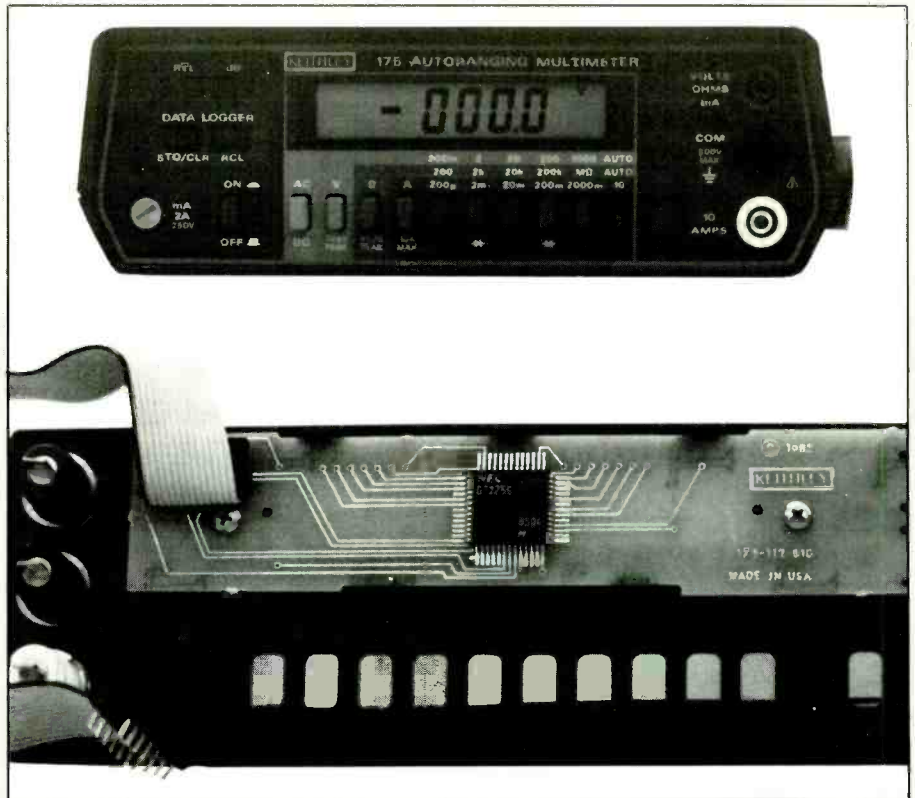
A 64-pin surface-mount LSI device is used for display drivers in a Keithley Model 175 DMM, saving 5 to 6 times the space that would be required for through-hole devices.
