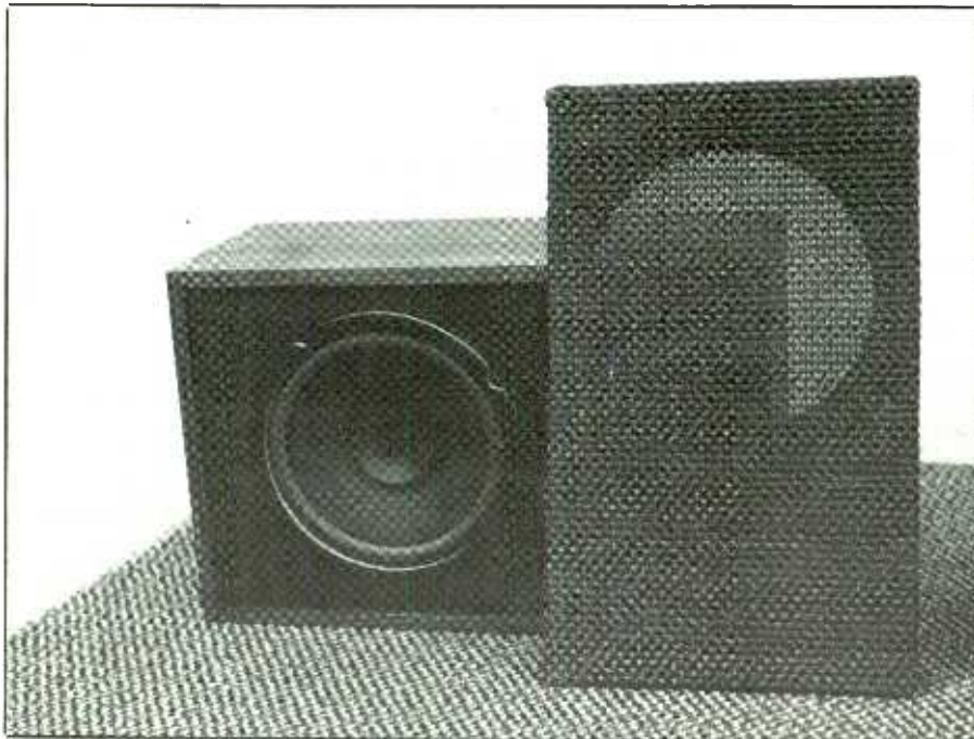
The grille for the speaker system consists of an open-weave cloth that is stretched on a 1/4"-thick frame and is held in place by friction.
