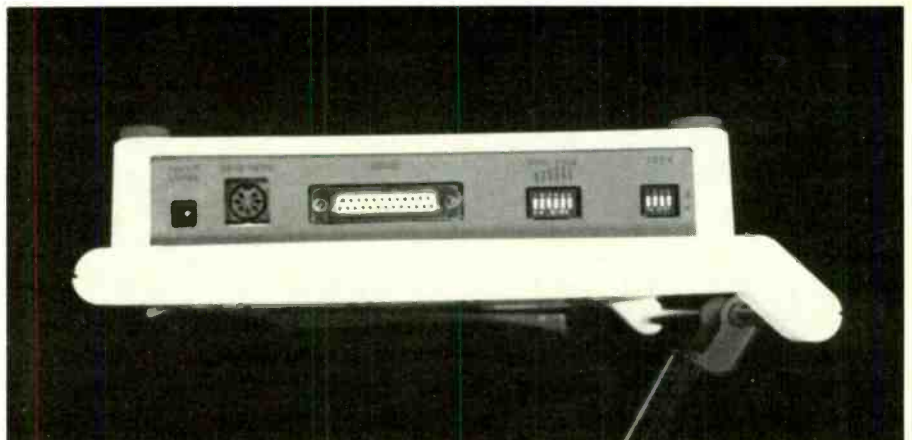
The rear edge of the tablet contains, from left to right, a jack for the power supply, a socket for the read head connector, an RS-232 I/O, baud-rate DIP selector, and the DIP selector for 10 or 12 pitch, modem Xon/Xoff handshake, internal beeper on/off and # or £ selection.
