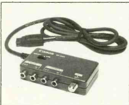
R-f unit has a vhf output and separate video/audio inputs and outputs.
