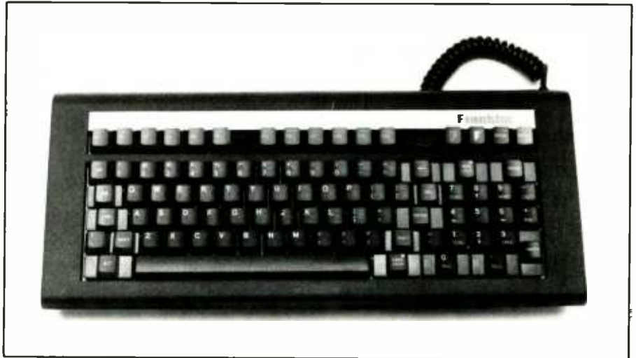
Franklin Ace 2000 keyboard features alphabetic, numeric, punctuation, special-character, 12 function, nine special editing, and numeric/cursor-control keys. LEDs are built into the Caps Lock and Num Lock keys.
