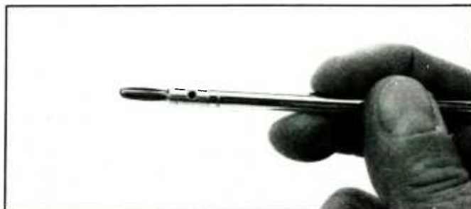
This telescoping antenna was salvaged from an old transistor radio. It is cross-threaded into a banana plug.
