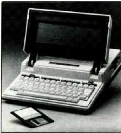
Tandy's Model 600 laptop computer has a 16-bit 80C88 microprocessor, a 16 by 80-character LCD display, 32K of RAM (expandable to 224K), parallel and serial ports, a 3.5" floppy-disk drive and firmware in ROM.
