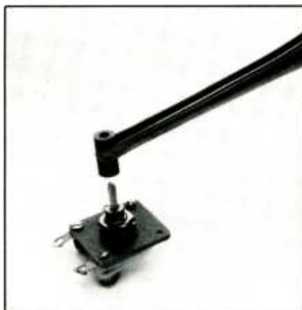
The specified tuning capacitor has a stub shaft originally intended for a tuning dial. You extend the shaft to accommodate a conventional knob by cementing a hollow spacer on the stub. A short section of toothpick in the stub serves as a centering device for the spacer.
