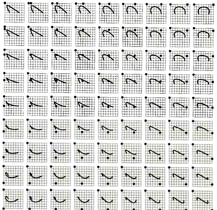
Fig. 3. This is a sample page from a cubic spline catalog. The dot is the first influence point, while the square is the second influence point.
