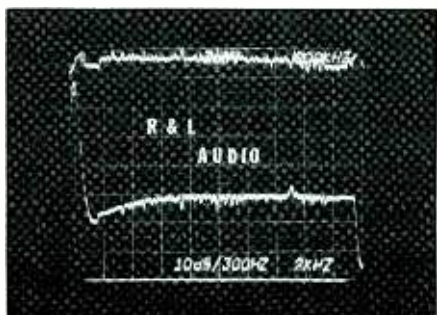
Right and left audio response to sine inputs; separation is 46 dB.
