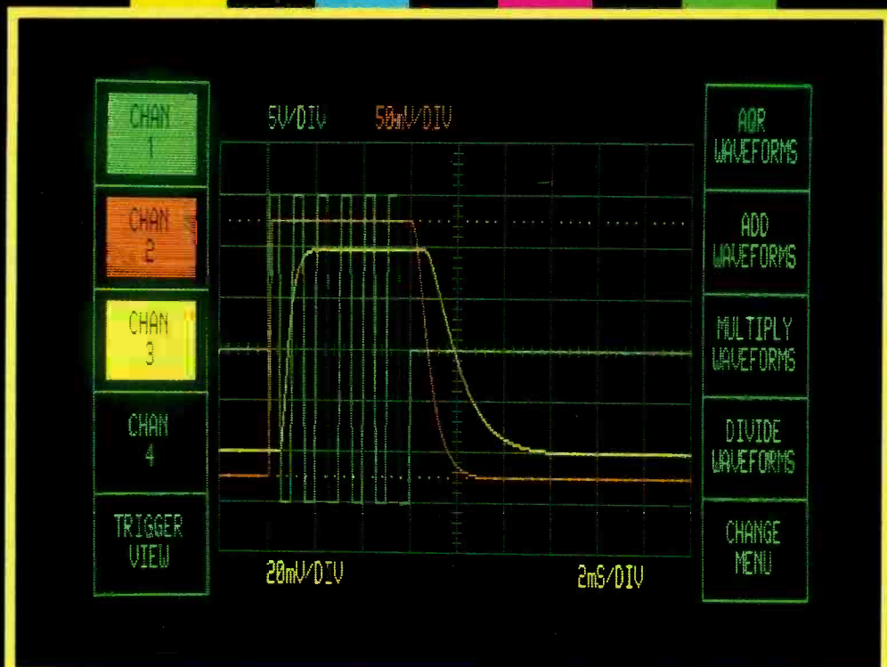
Fig. 1. An oscilloscope trace with the liquid-crystal shutter displays three separate colors with a monochrome cathode-ray tube for backlighting.
