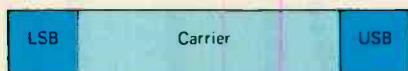
Figure 2 Power distribution in the AM signal. Each sideband is a mirror image of the other and each contains 16.6% of the total power in the signal.
