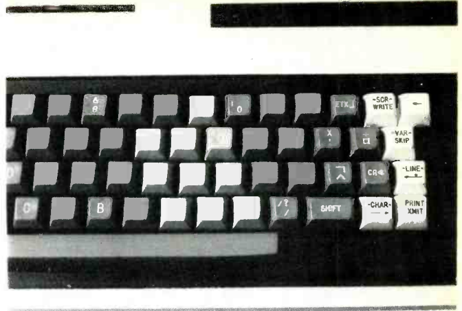
A computer terminal's keyboard has several added keys you won't find on an ordinary typewriter. Otherwise it's similar. An important key always used is the CR or Carriage Return key, shown at right.
