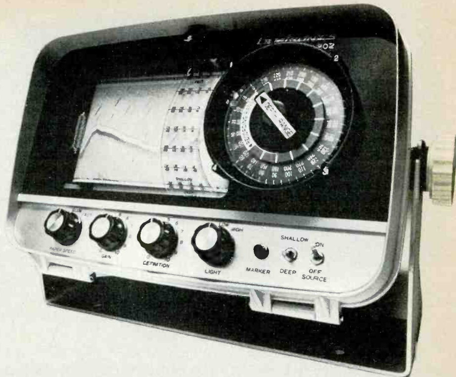
The Gemtronics GT-1202S is claimed to be one the most sophisticated flasher-recorders available. With an overall depth range of 480 feet, its special 30-foot range makes it ideal for bass and other shallow water fishing.
