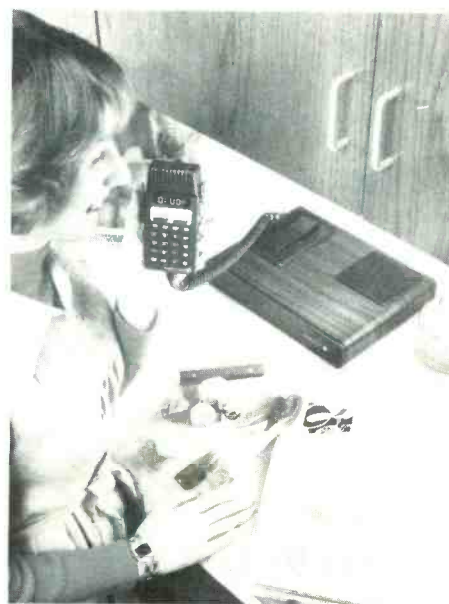
SSB CB mobile radio, above, and base station, right, by Texas Instruments, have microcomputers built in. All controls are in the handset/microphone.
