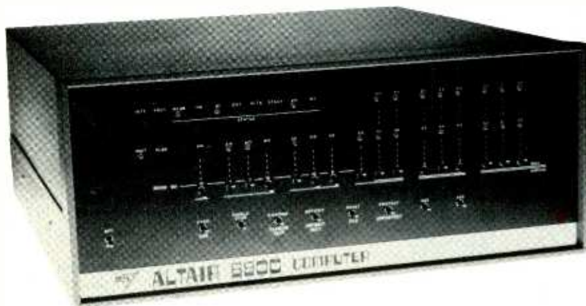
Here's where it all started a couple of years back. MITS Altair 8800 was the first micro-computer sold to hobbyists.
