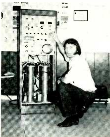
Joe deCourcelle, K3OBU, operates this repeater near Philadelphia. Bottom half of the cabinet is filled with duplexer.
