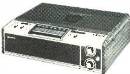
Sony's V Cord II uses higher tape writing speed for a sharper picture.
