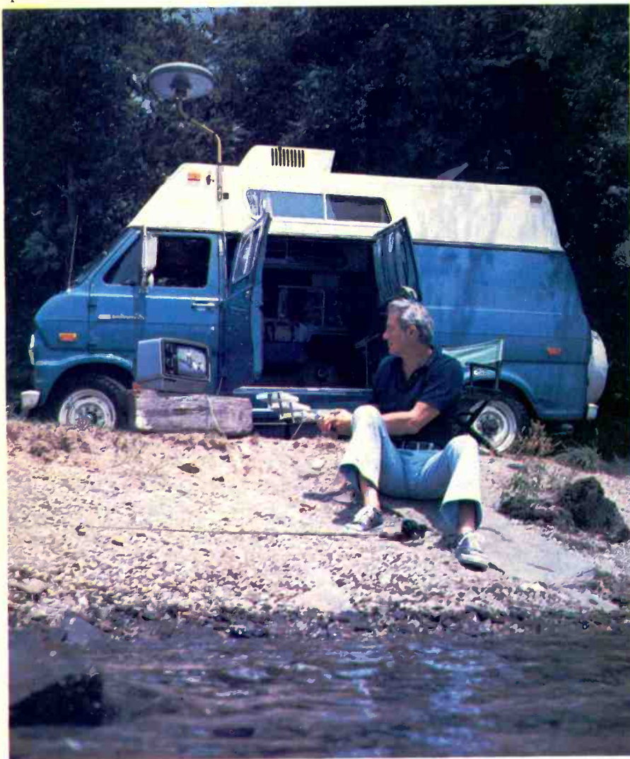
When the fish aren't biting, Charlie Myers can watch the ball game on tv. Charlie mounted on his camper a flying-saucer shaped RCA tv antenna. The Mini State antenna is powered by the 12-volt battery in his recreational vehicle. A hand-held remote control lets him point the antenna electronically for the best tv signal. It also operates from 120-volt ac house power when Charlie is home.
