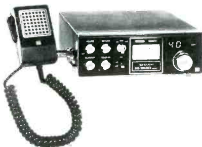
SSB CB mobile radio, above, and base station, right, by Texas Instruments, have microcomputers built in. All controls are in the handset/microphone.
