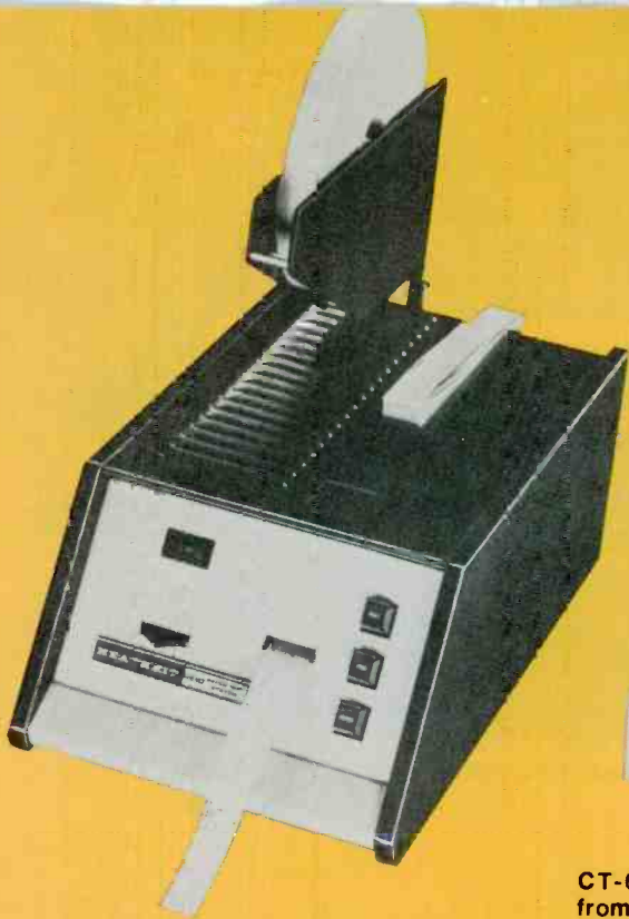
Heath H-10, above, is a different input/output device which reads holes punched in paper tape and punches new tape.
