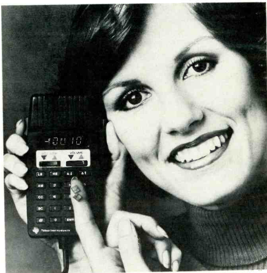
Two! That's right, two microcomputers smaller than the tip of her fingers talk to each other in the Texas Instruments CB. One is in the microphone; one in the radio. They keep a constant housekeeping watch on the inner workings of the set plus do such extra chores as fine tune the receiver for off-channel signals.
