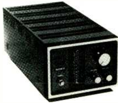
Sony pulse-code modulation box takes audio, which is an analog signal, and changes it to a digital signal for better storing on tape. It reconverts, digital-to-analog, upon playback.
