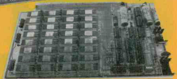
Altair 680b, left, by MITS, is smaller than the 8800b but popular because it does most of what the 8800 will do. Circuit board, below, plugs into 680 to give it a very large 16K memory.
