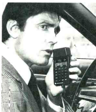
SSB CB mobile radio, above, and base station, right, by Texas Instruments, have microcomputers built in. All controls are in the handset/microphone.
