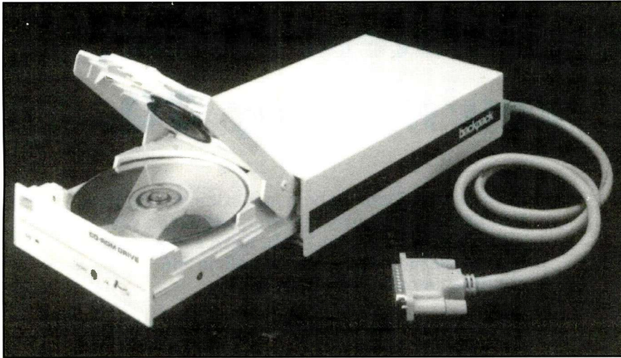
MicroSolutions Backpack CD-Rom drive plugs into a parallel printer port and features pass-through for normal printing.
