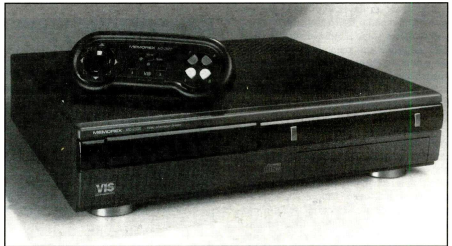
Tandy/Memorex MD-2500 VIS player looks innocuous as a consumer-level device, but it's really a DOS-based PC in disguise, capable of playing audio CDs and CD+G discs a proprietary VIS format but not Photo CDs.
