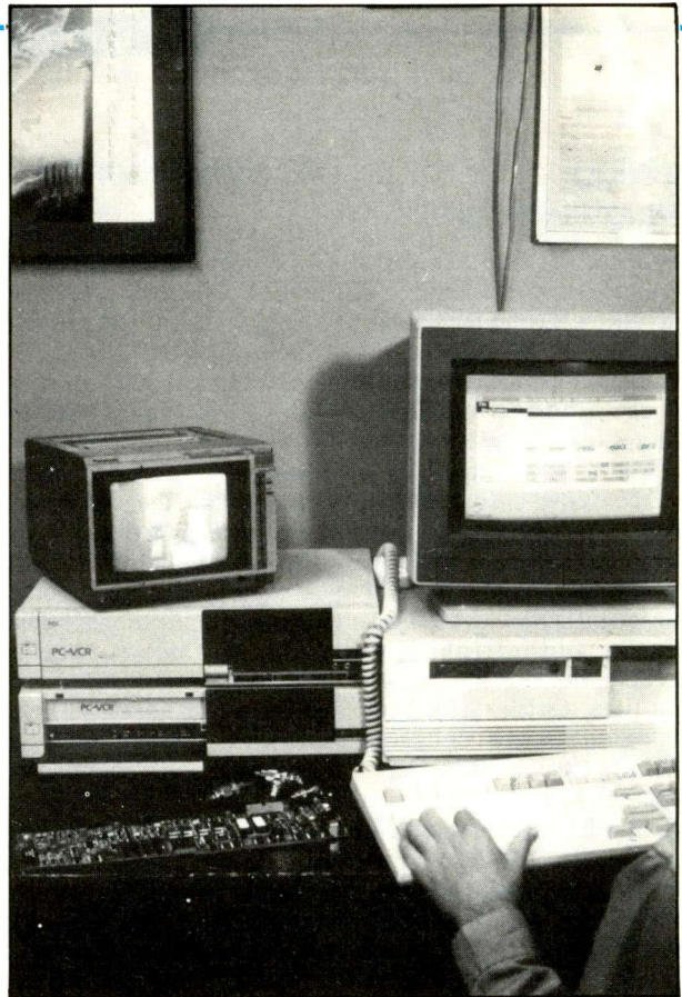
Two NEC PC-VCRs interfaced to a 386 computer afford the ultimate in computer-controlled editing and scene transfer.
