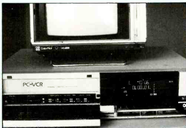
View of NEC PC-VCR with front panel open to show the cassette access door and keypad control section.
