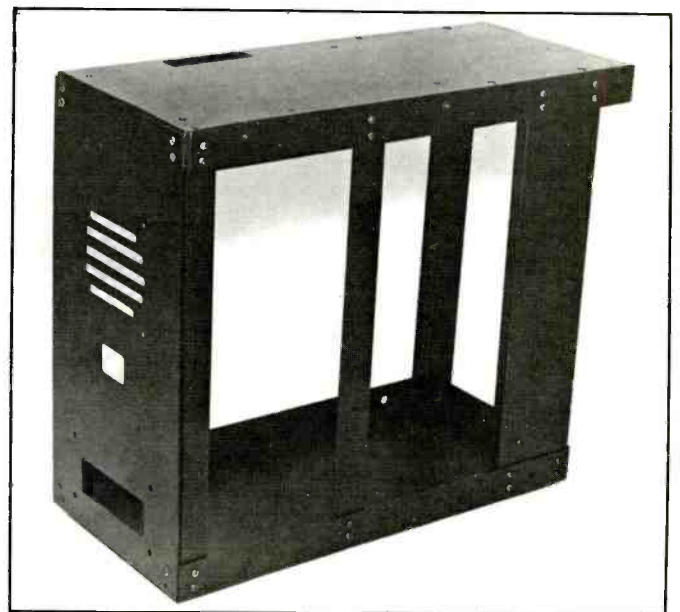
After securing the motherboard brackets to the bottom shelf, secure the top shelf to the ends of the upright brackets.
