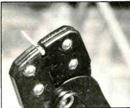
Photo 4. Crimper is used to make a pin fit into its jaw slot.
