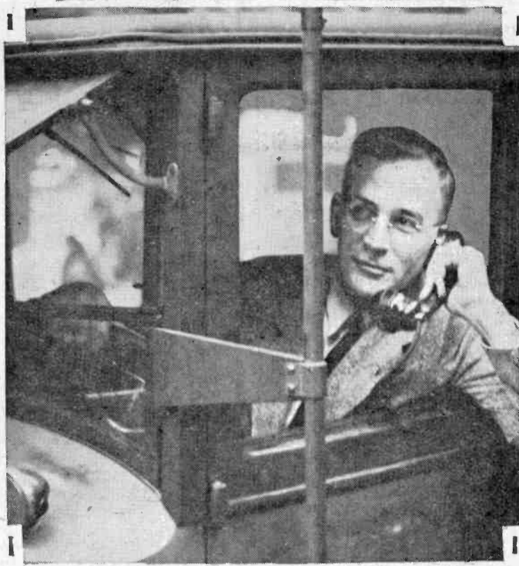
SAM CURTIS, Boston radio engineer, with his two-way radio equipped car that attracts much attention. The telephone is connected with a radio apparatus behind the driver's seat.
