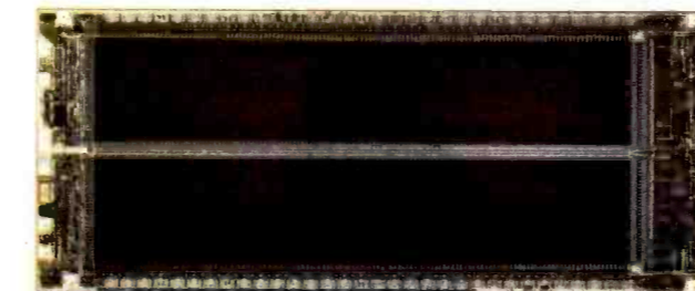
64 kbit dynamic RAM; 3 \mu m NMOS; 135000 transistors; 3.0 x 7.1 mm (STC).
