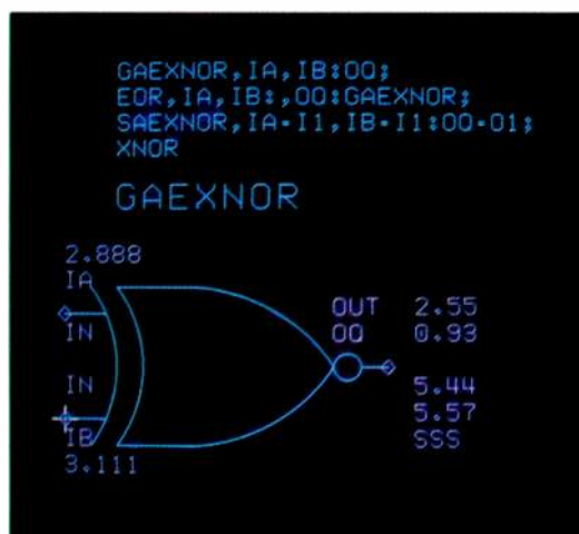
Figure 2 A sample logic symbol showing the physical attributes attached to the symbol and pins.
