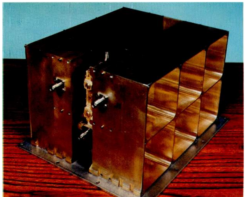
Engineering development model of the triplexer for the global positioning satellite.
