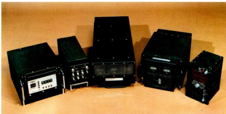
Navstar receiver developed by Standard Telecommunication Laboratories. From left to right the units are the program loading unit, RF front end unit, channel unit, and control and display unit.
