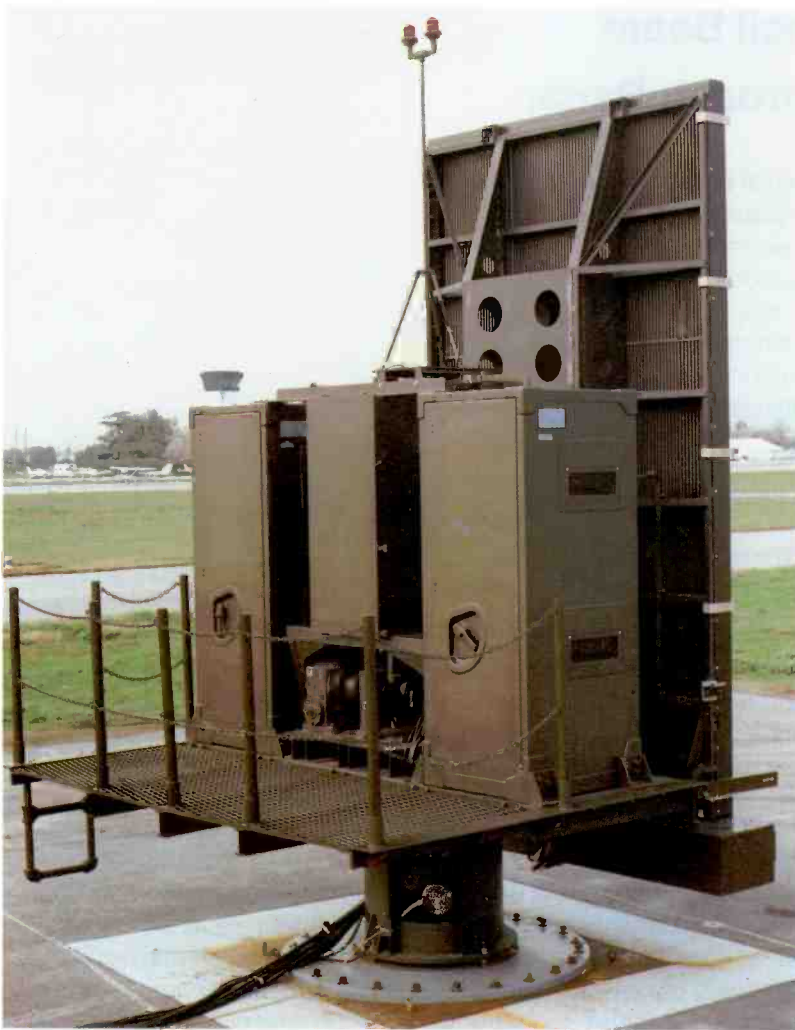
Radar set group of the PAR-80. The dual receiver-transmitter cabinets are located on either side of the turntable-mounted platform with the scan programmer and elevation drive between them.
