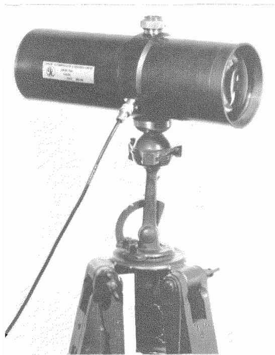
Figure 3—Wide-band optical data-link transmitter for use over paths that are inaccessible by more-conventional means.
