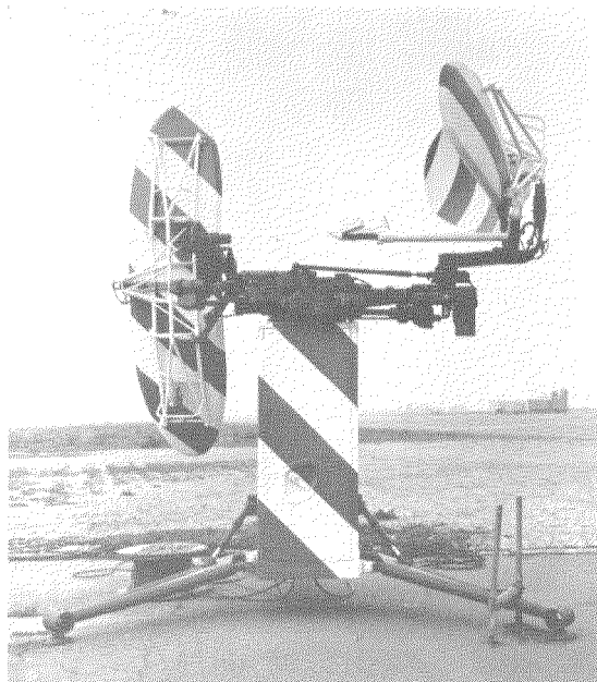
Figure 4—Quadradar installation for surveillance, final approach, height finding, and air-traffic taxi information.
