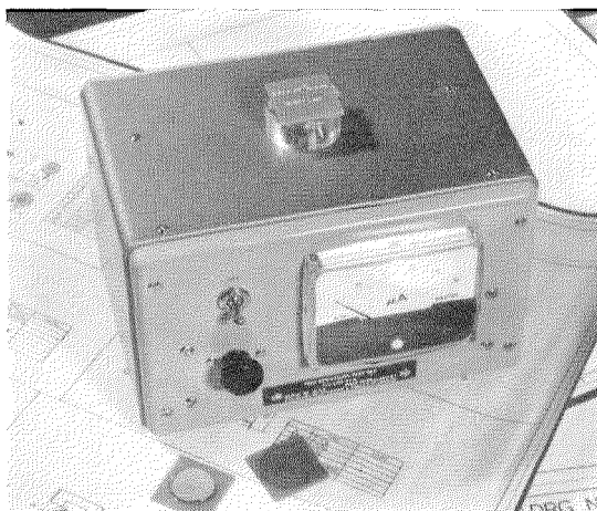
Figure 10—This test set measures the resistivity of thin slices of semiconductor material by its damping effect on a lightly loaded tuned circuit.
