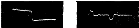
Figure 3—Oscillograms showing at the right the 3.5-microsecond limited pulses resulting from the action of the short-circuited delay line on the long pulse shown in the left part of the picture.
