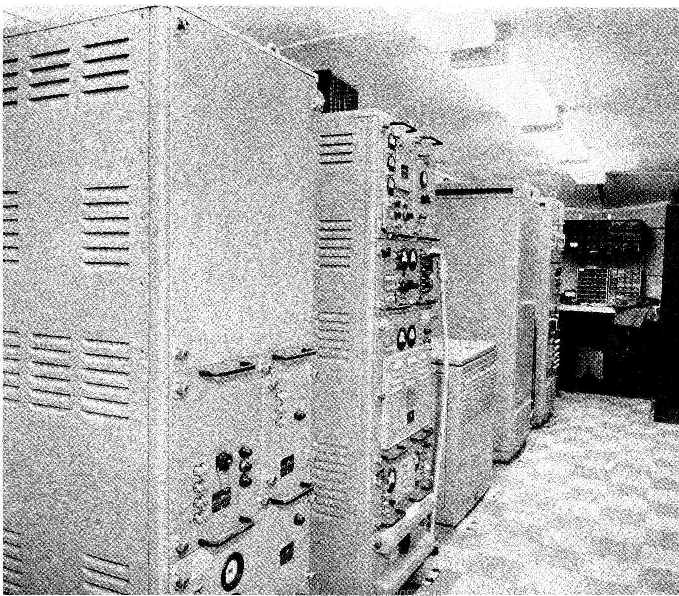
Figure 22—One of the trailers houses a standard tacan beacon in the two cabinets at the left and digital storage, coding, and control units for the data link.
