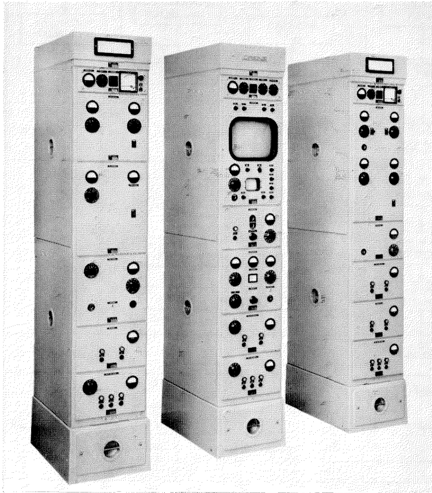
Figure 1—These 3 racks contain the equipment for a terminal station.
