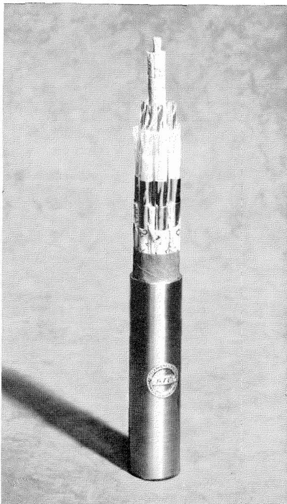
Cable containing 8 polythene-insulated video-frequency pairs. There are also 8 star quads and 14 pairs in the interstices.
