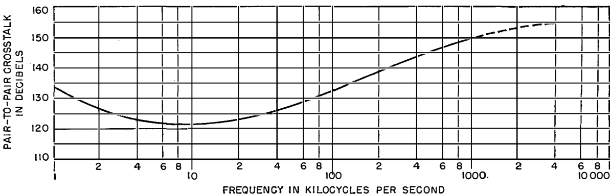
Typical pair-to-pair crosstalk curves plotted against frequency.
