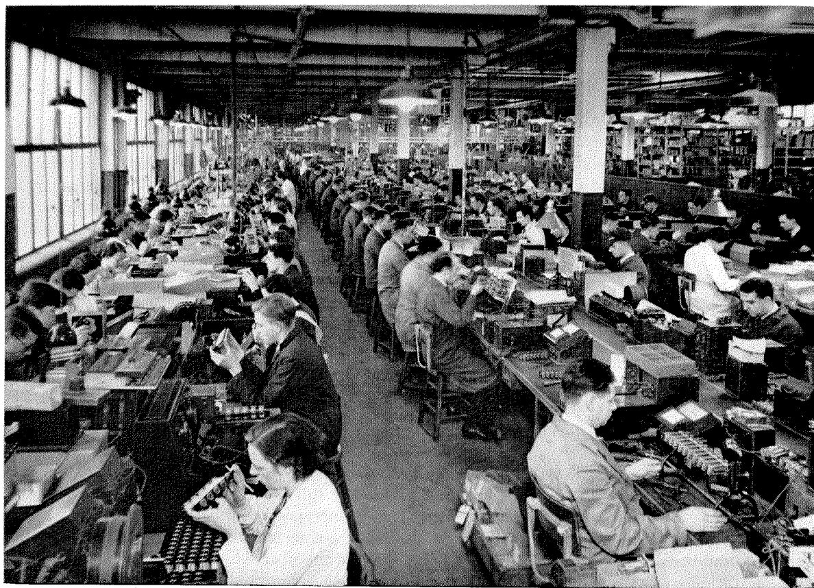
Figure 14—Adjustment of relays at the Antwerp factory of Bell Telephone Manufacturing Company.
