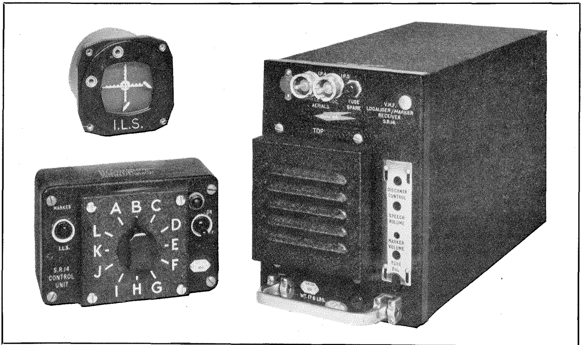
Figure 1—The receivers are in the large case, with the control unit at lower left and cross-pointer indicator above it.
