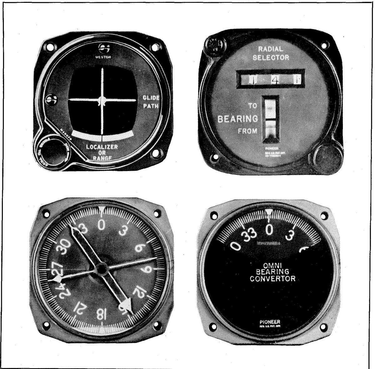
Figure 6—Various indicators used with the receiver. At top are the flight-path-deviation indicator and omnibearing selector and below are the radio-magnetic indicator and omnibearing convertor.
