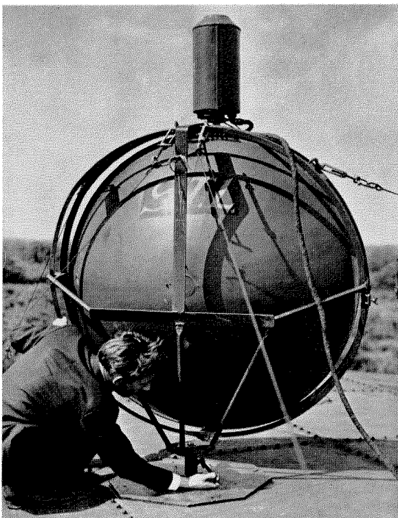
The transmitting circuits are enclosed in the weather-proof cannister above the 4-foot paraboloid, which is being aimed at a distant receiver.
