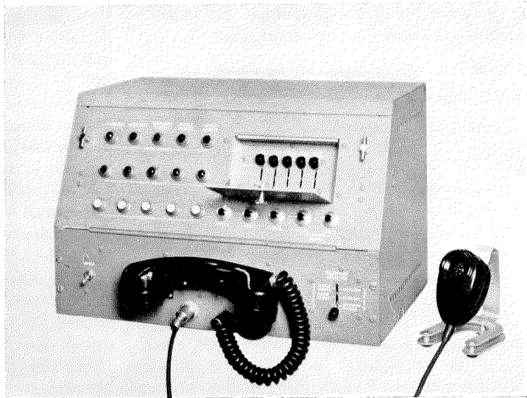
Figure 5—Control unit. Switches and alarm lamps are on the panel; the microphone for simultaneous voice is at the right. The telephone handset is for communication with other parts of the system.
