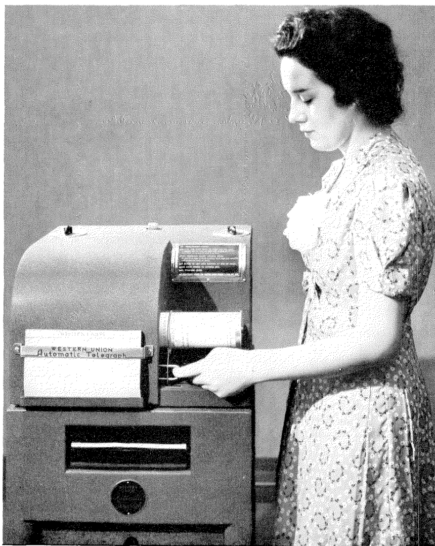
Figure 1—Telefax transmitter-recorder with optical scanning.
