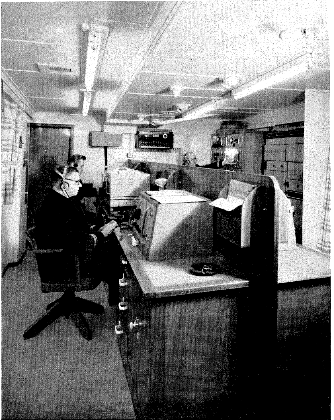
Radio receiving room and operating positions aboard R.M.S. Caronia. The single-sideband radiotelephone receiver and terminal equipment are in the far corner of the room.
