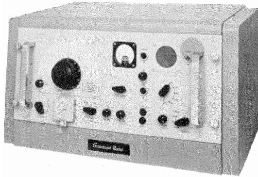
Figure 16— R.V.9. medium- and high-frequency receiver.
