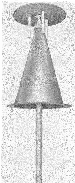
Fig. 5—Discone antenna for cutoff frequency of 90 megacycles.
