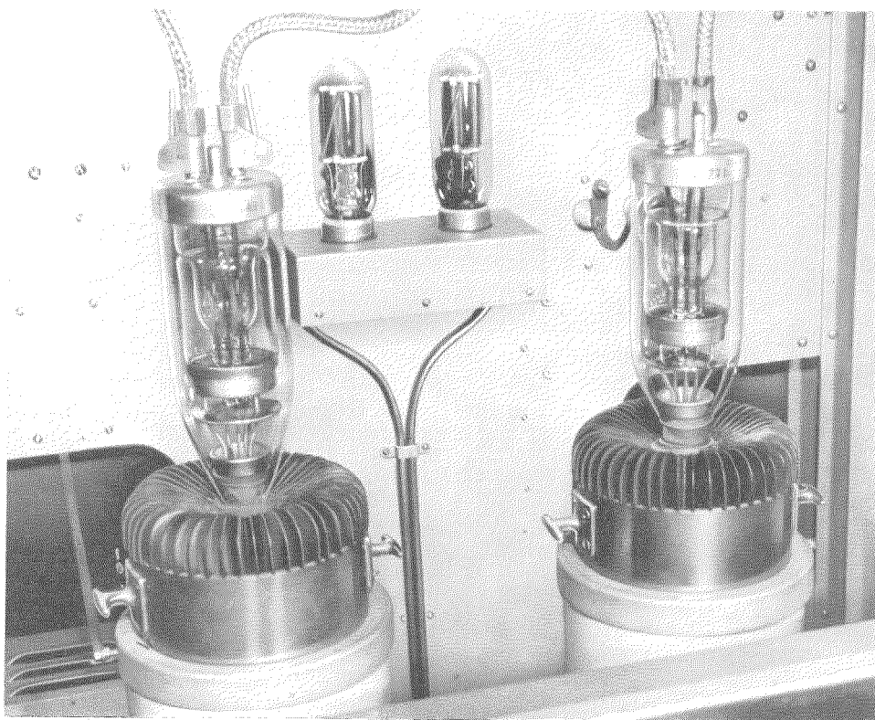
Fig. 6—Air-Cooled Modulator Tubes of the 5-Kilowatt Auxiliary Transmitter.
